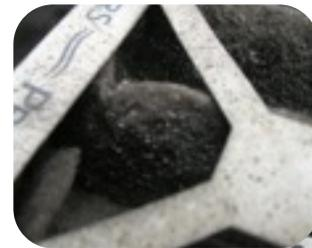
*Moisture damage and microbial growth on pleated filters.*
